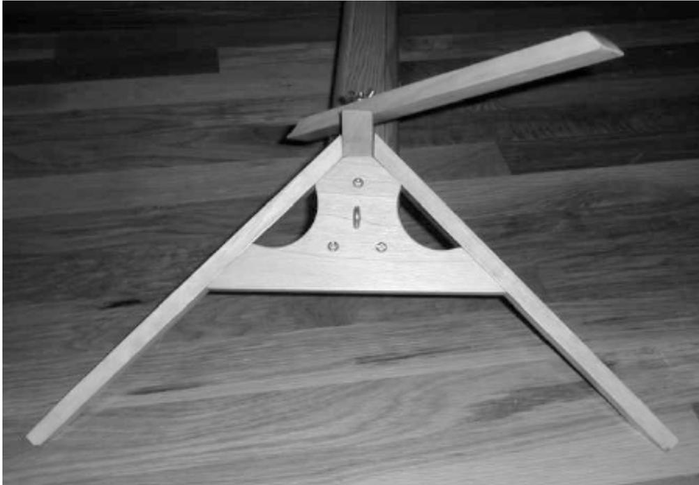
Check alignment of rear bracket against back of neck. Extend guideholes through neck into rear bracket, then enlarge them in the neck to  $9/64$ ". Countersink these holes and attach neck to rear bracket with 2 #6 2" phillips flat-head wood screws.
