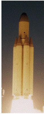
The Conestoga 1620 was developed by Space Services Inc. as a small satellite launcher. In 1990, EER purchased SSI and continued development. However, its only launch to date (in 1995) ended in failure due to a hydraulic actuator problem. Correcting the problem would require additional money, which does not appear to be forthcoming. At this writing, it appears the Conestoga's first flight was also its last.
